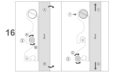
Eccentric screw 2 adjusts side inclination ( A and B)
