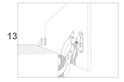
Apply the doors on mechanism as per Pict.13.
