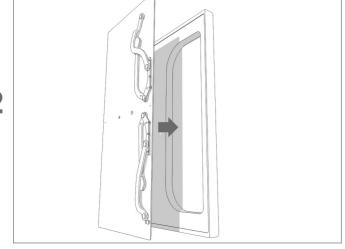
Place mechanism on cabinet and test out that it's "free" on motion.
