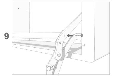
Fit the connection and tighten screw to lock it firmly.
