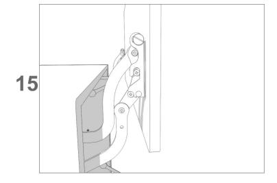
After to place the door and after to insert the screws as up as down, adjust the door as per *Pict.16*.
