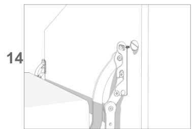
Insert the screws for the fit of the door with no tightening them.
