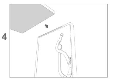
Place and fit the upper cabinet's board so that it constrains and it stop eventual mechanism's movements.
