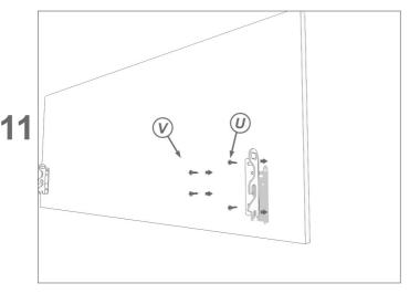
Place the plates on the door as per technical card and insert the external screws  $(\textbf{\textit{U}})$  with no tighten them to allow the adjustment of the door.
