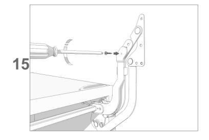
Mount swing system on mechanism and tighten it with screw as per picture.
