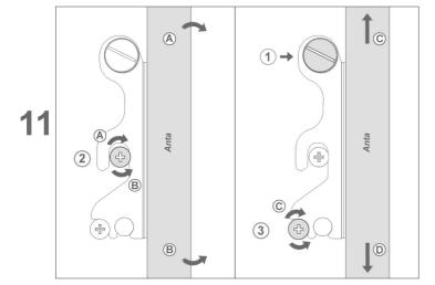
Eccentric screw 2 adjusts side inclination ( A and B)
