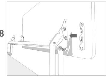
Place door with plate mounted on mechanism as per picture.
