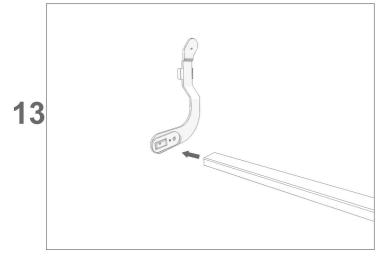
To fit swing system on mechanism mount mechanism as per *picture 4* then fit connection rod to the two swing fittings as per picture.
