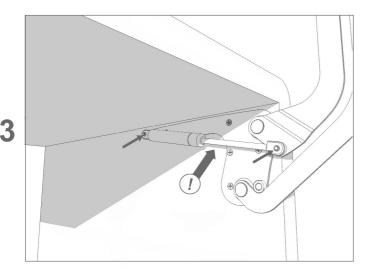
Place piston with "open" mechanism as per picture (ATTENTION: piston mobile rod has to be turned downwards)
