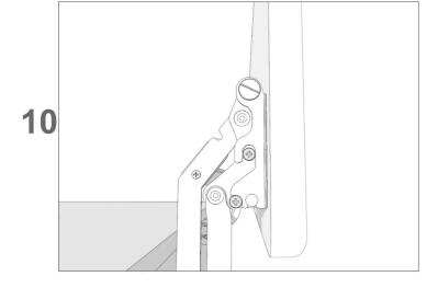
Adjust door with screws as per picture 11
