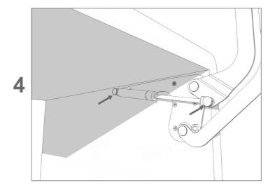
Fit splits on pins where piston has been fitted. Then repeat this operation for the other cabinet side with the other mechanism element.
