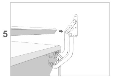
Fit connection to mechanism on both sides as per picture. Connection rod length is given by cabinet inside dimension less 31.5 mm with +- 0.5 tolerance.
