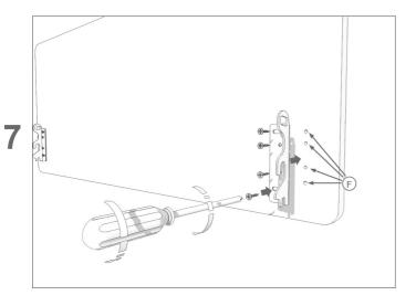
Drill cabinet door as per technical card (F) fit plates and tighten them firmly.
