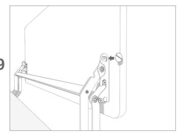
Insert clamping screw without tightening it to allow adjustment.
