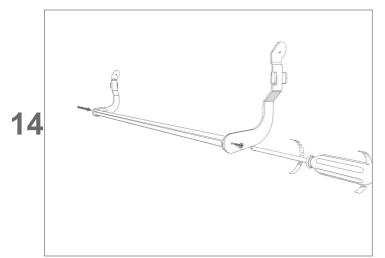
Insert screw to tighten cabinet as per picture.
