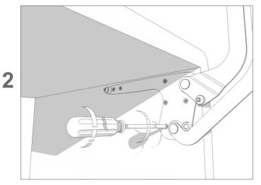
Place mechanism on cabinet and tighten screws to lock it firmly.
